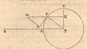
If P T equal the addititious force, then the ablatitious force equals 3 P K, for P K : P T : : sin.  $\theta$  : (1 = r),
